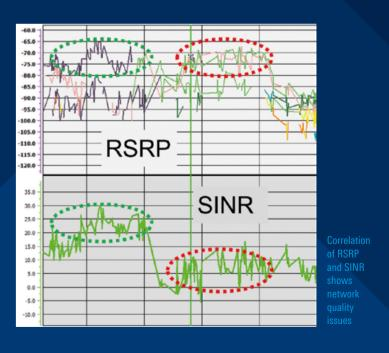
A network scanner together with QualiPoc Android or R&S®ROMES4 identifies and provides an overview of all received signals/cells from multiple technologies in multiple frequency bands by multiple operators within seconds. This automatic channel detection (ACD) delivers a quick overview of spectrum usage and indicates mobile network quality.
