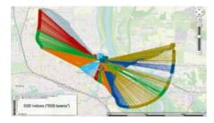
R&S\*ROMES4: outline color represents the best SSB index beam received by a scanner on the drive test route
