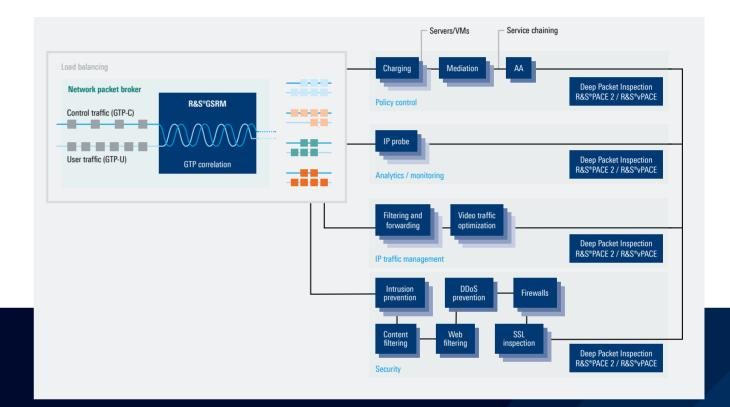
The deployment scenario shows the GTP correlation module R&S°GSRM and the DPI engines R&S°PACE 2 and R&S°vPACE embedded in a network architecture.
