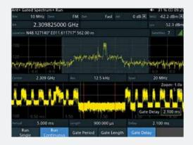
The unique parallel time and frequency domain analysis on the R&S\*PR200 allows the user to keep an eye on the gate configuration without losing sight of the spectrum signal
