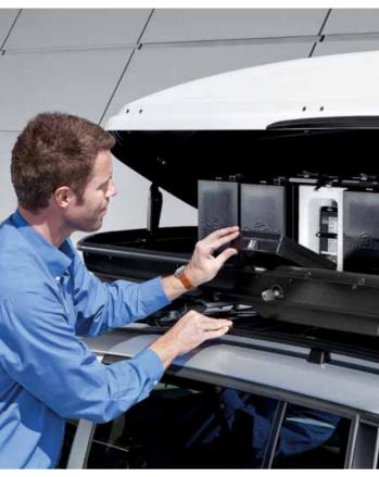
Vehicle roof box setup: TCMs can be installed in the specifically designed Vehicle roof box (VRB) and connected to Benchmarker II. The VRB can contain up to 16 TCMs (measurement channels) and ensures uniform RF and temperature conditions. The roof box and the IP65 rated cable duct for the cable entry into the vehicle can withstand any weather conditions.
