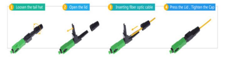
Note: The fiber must be cut flat, otherwise the connector will be damaged.
