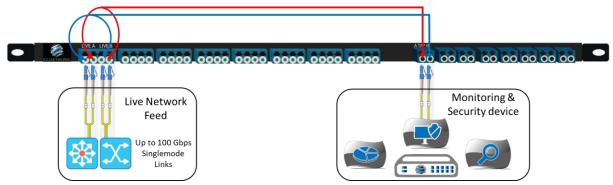
The TAPstack connects to the live network using LIVE A & B ports, and mirrors traffic to the TAP ports, for inspection by a network analyzer, monitor or security device.
