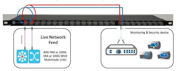
The TAPstack MTP TAP is designed to simplify the Multimode cabling infrastructure for 40G/100G. Each TAP requires an MTP Y cable that splits the input feed from the TAP port to two ports on the network packet broker or on the monitoring tool.
