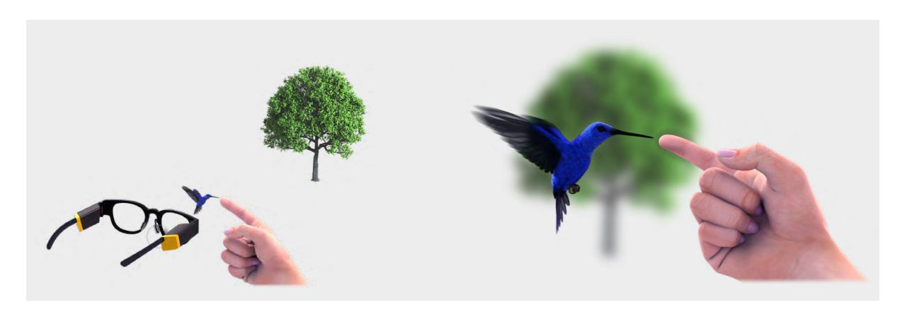
CREAL's technology displays light-field images at any focal distance ...
