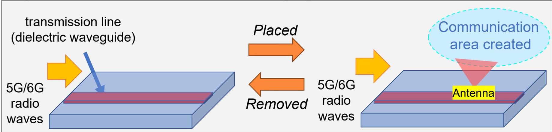
The antenna, a small piece of plastic, causes strong radio waves to leak from the cable, creating a local communication area.
