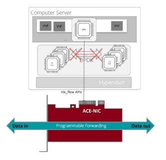
The result is optimized high-performance data forwarding on programmable, futureproof hardware. ACE-NICs provide deterministic throughput of up to 100G and sub-3µs latency without CPU intervention, freeing up those resources for running the control functions and applications for which they were designed, as well as saving physical space and power. The result is to save up to 80% on both operating and capital expenditures.
