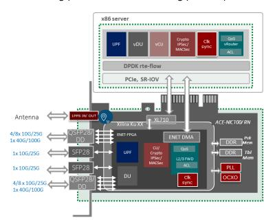
ACE-NIC50 and ACE-NIC100 SmartNICs with 10/25/40/100 Gigabit Ethernet connectivity, built using the FPGA-based Carrier-grade ENET Flow Processor technology, provide best-in-class performance and an unsurpassed feature set of acceleration and forwarding offload for 5G, telco, and enterprise NFV. Built to accelerate cloud and Multi-Access Edge Computing (MEC) infrastructure, the ACE-NIC family is optimized for carrier-level quality of experience, performance, and power at scale.
