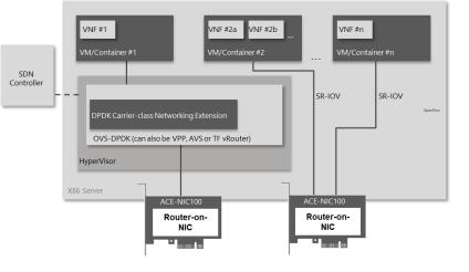
offload that effects multi-purpose smart hardware that accelerates performance, improves agility, and reduces expenses. ACE-NIC includes several features which enable it to offload NFV, such as L3 routing, encryption, IPSec, 5-tuple capabilities, deep packet inspection, and others.
