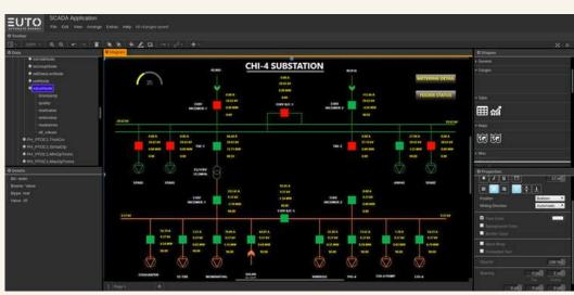
Cloud-based software product for developing configuration-level IoT and SCADA automation applications nocode with standard protocol support.
