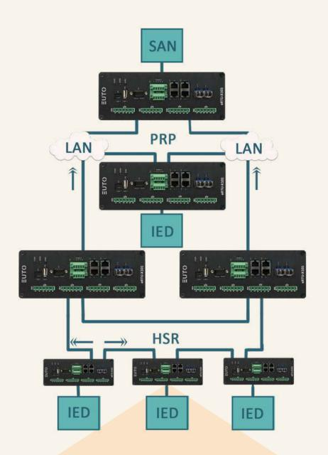
HSR/PRP can be applied from configured fiber optic and copper ethernet ports to supply zero recovery time on network faults.
