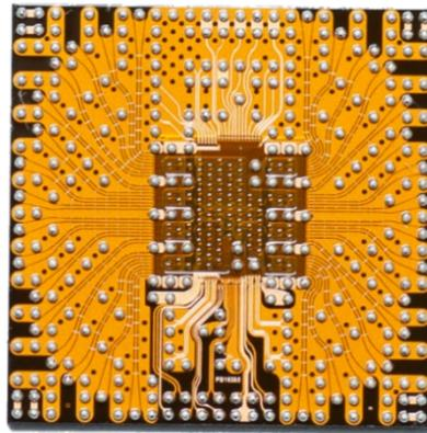
The license free 60 GHz band enables new opportunities to operators where high data rates and range are of essence. The Sivers Semiconductors TRXBF01 supports the full frequency range from 57 to 71 GHz with speeds up to 7 Gbit/s and beyond, long-range. The perfect choice for unlicensed 5G.
