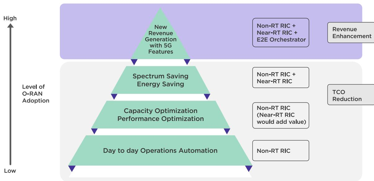
Figure 4 – RIC use cases: A high level classification and calibration with O-RAN adoption
