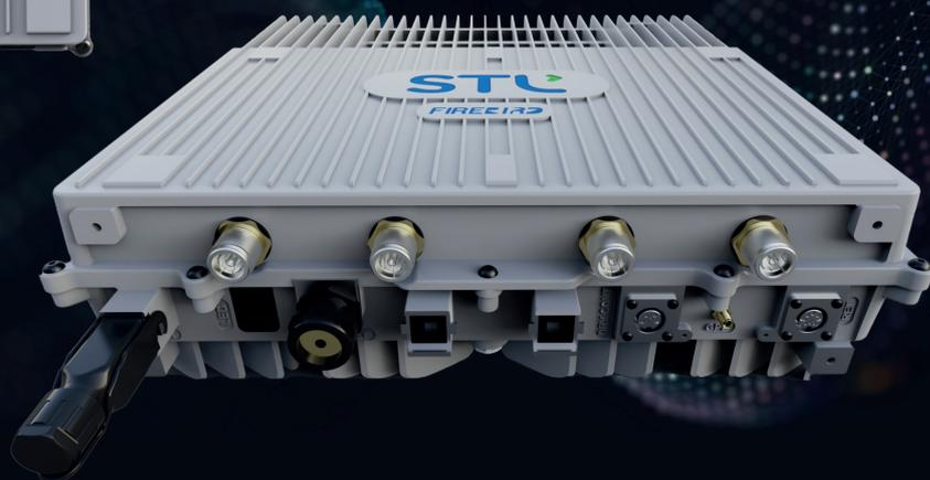
STL Firebird is a portfolio of multi-band multi-RAT FDD & TDD macro open radio units (O-RUs) available in different bands. These carrier grade macro O-RUs are compliant with 3GPP Release 15 and can be upgraded to Release 16 through software updates. These standardized O-RUs works seamlessly with O-DU from any vendor to form the gNodeB and supports the delivery of high-speed data, mobility, seamless voice and broadcast services.
