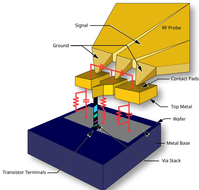
Figure 1. The back-end-of-line (BEOL) parasitic circuit elements and probe interconnect resistances and capacitances increase the uncertainty of on-wafer measurements and impact device model accuracy.
