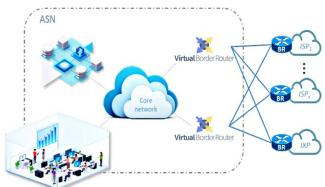
The 6WIND VSR implements traffic splitting and balancing between multiple links to optimize packet flow, reduce latency and enhance connectivity.
