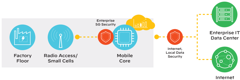
Figure 2: Reference architecture depicting security positioning over enterprise 5G networks
