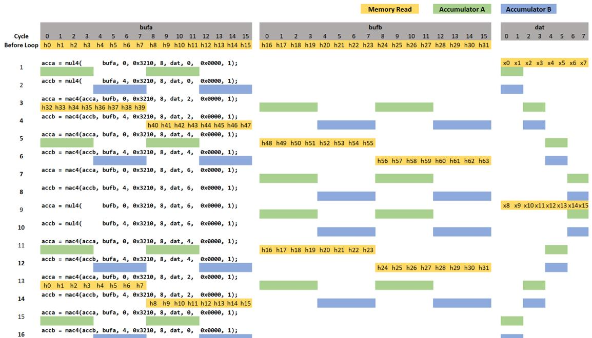
The kernel `bf8x8_mid` reads the partial summation from the previous AI Engine before starting the first MAC operation. In the following C code, the intrinsic `getc_scd()` loads the data on the cascading bus into an accumulation register, and the intrinsic `mac4()` resumes the accumulation without wasting any clock cycles.
