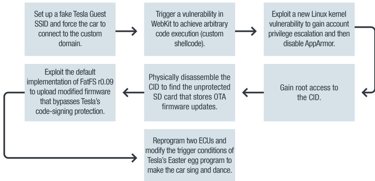
Figure 27. The attack chain of the Tesla Model S remote hack of 2017
