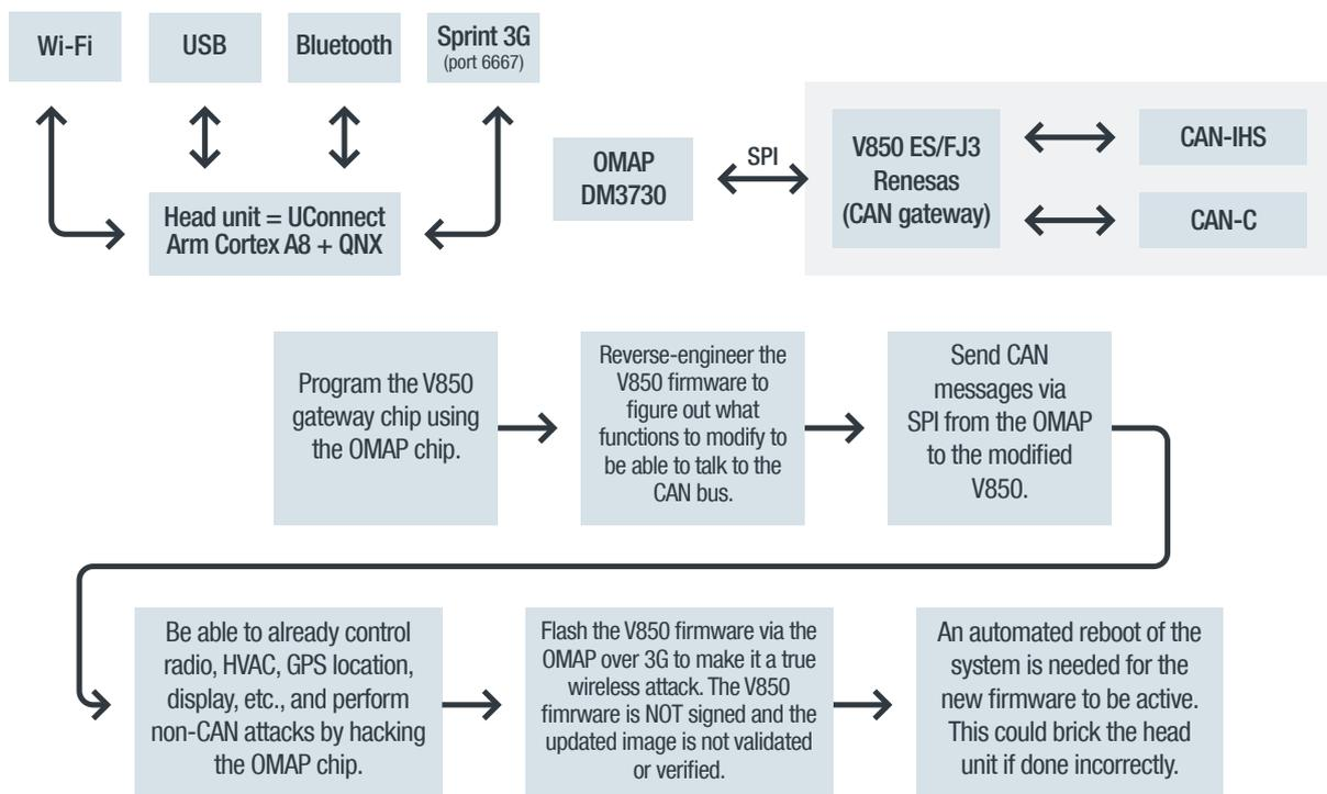
Figure 25. The attack chain of the Jeep Cherokee remote hack of 2015
