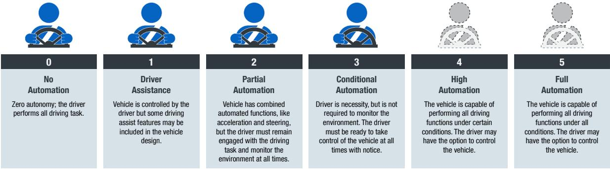
Figure 2. Society of Automotive Engineers (SAE) automation levels
