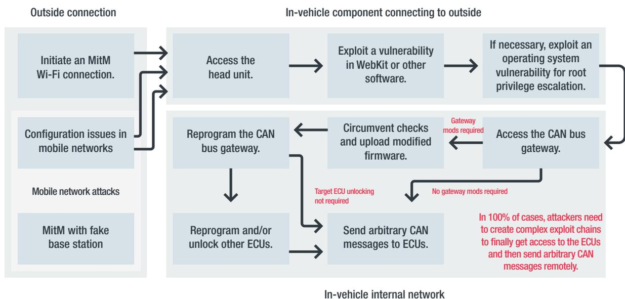
Figure 7. A generalized remote hacking attack chain based on the featured remote attack case studies
