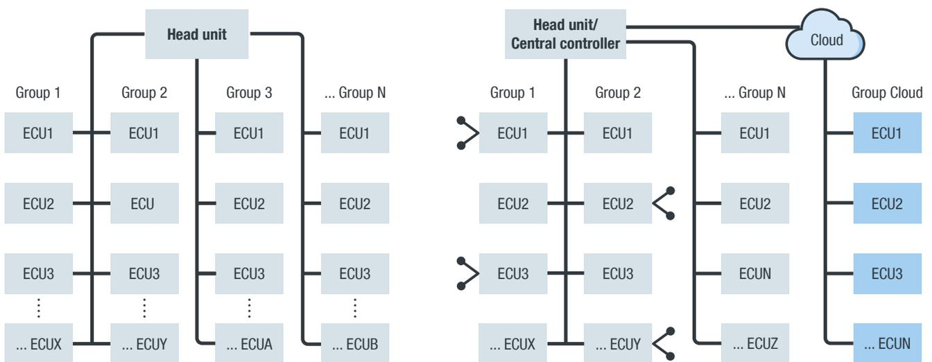
Figures 10. Car E/E architecture today (left) versus cloud-based car E/E architecture (right)
