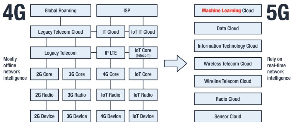
Figure 8. A side-by-side comparison of 4G and 5G networks for connected cars
