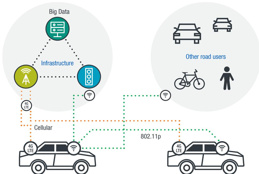
Figure 29. A side-by-side comparison of IEEE 802.11p and cellular connectivity for connected cars<sup>160</sup>
