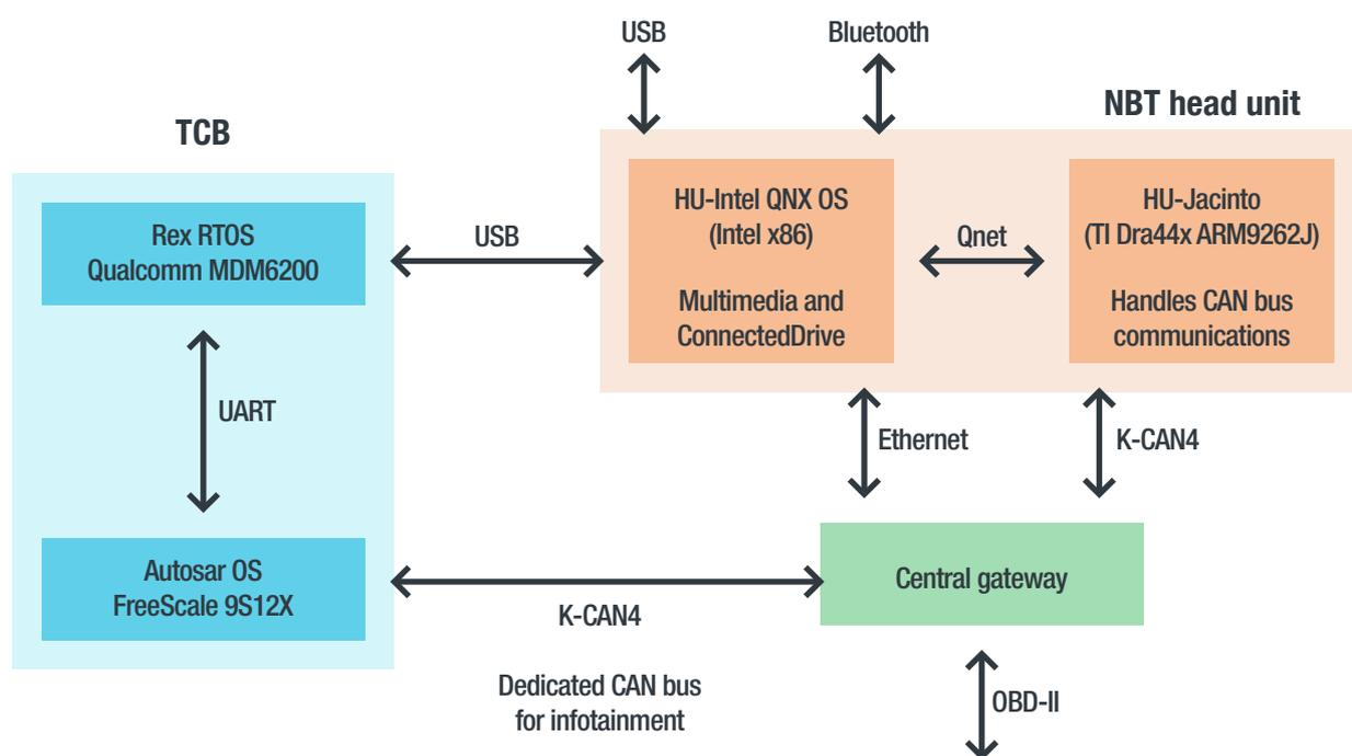
Figure 28. The attack chain of the BMW remote hack of 2018
