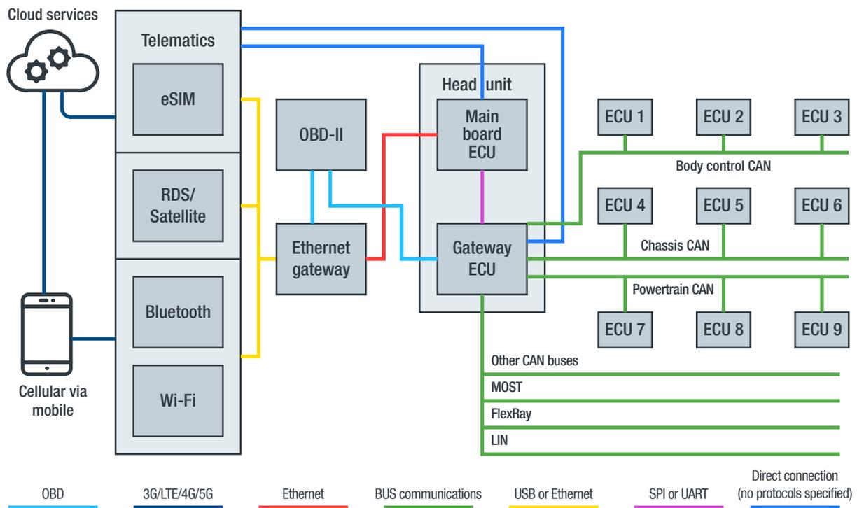
Figure 6. A theoretical visualization of a generic network architecture for a modern-day connected car
