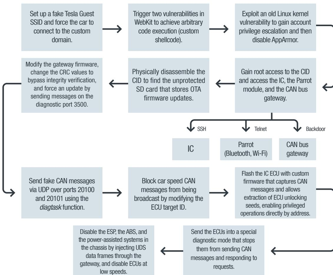
Figure 26. The attack chain of the Tesla Model S remote hack of 2016
