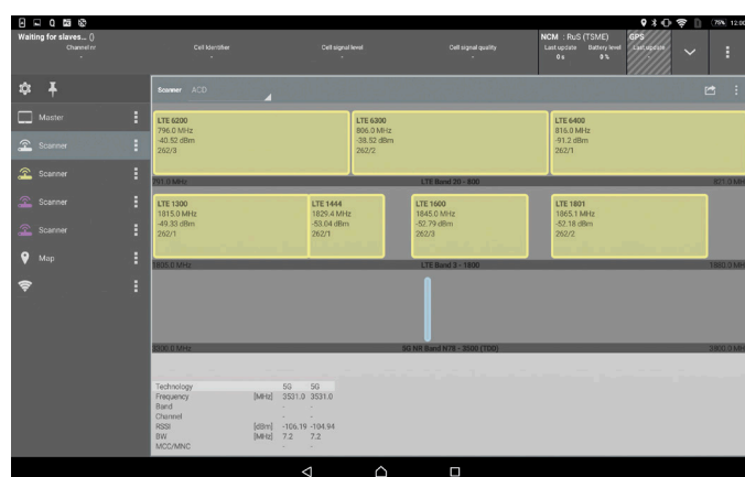
Fig. 8: Automated channel detection (ACD) showing bands 3, 20 and n78
