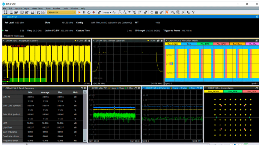
Analysis of a generic OFDM signal with R&S®VSE-K96.
