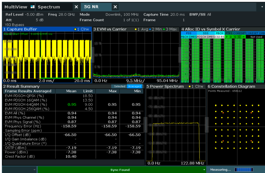
Analysis of a 5G NR downlink signal with R&S®FSW-K144.
