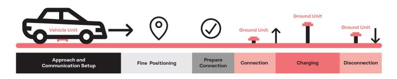
The sequence of events involved in wireless EV charging, which requires a wireless communication channel between the charging station and the vehicle.
