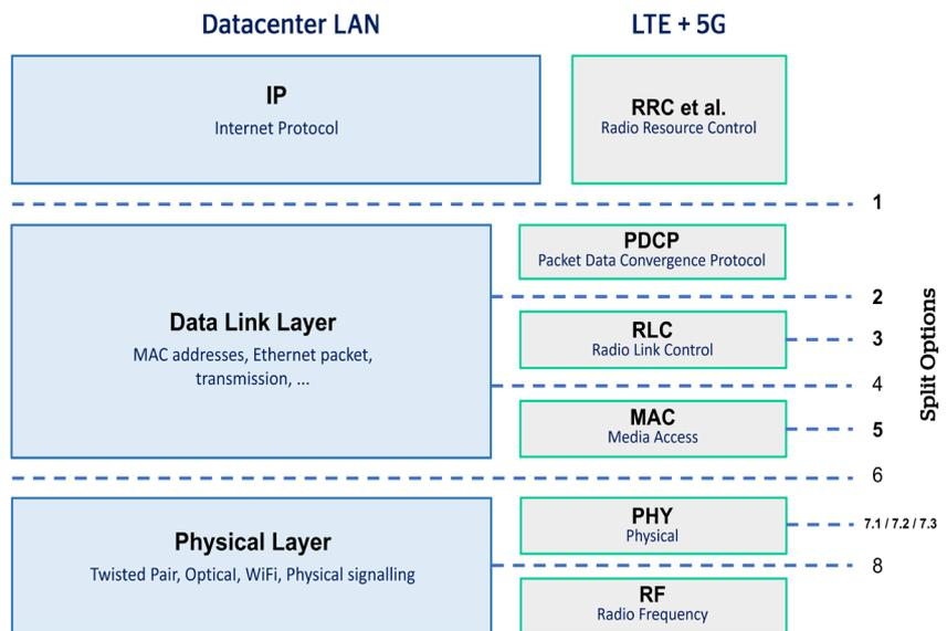
Figure 1: Datacenter LAN and LTE+5G RAN network stacks - a comparison
