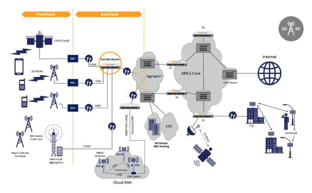
The OcNOS-SP-CSR solution is a smart converged integrated access platform which enables Service Providers to deliver next-level business and entertainment experiences and it comprises of the following core components:
