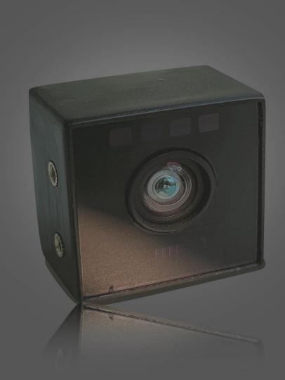
Solid-state ToF LiDAR Sensor
