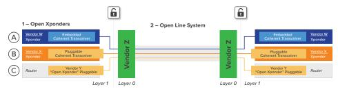
Figure 1: Open optical networking requirements 1 (open Xponders) and 2 (open line system)
