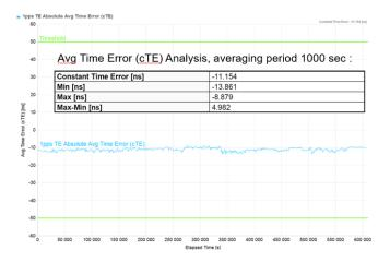
Figure 17: OTC2.0 time error of 11 ns after 500 km over six DWDM spans and seven timing hops
