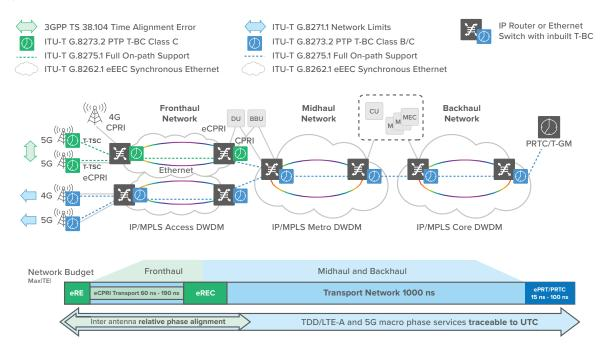
Figure 9: Delivering 5G-quality synchronization across the transport network
