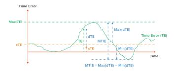
Figure 5: Maximum time error relationship to constant and dynamic time errors
