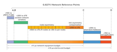
Figure 4: G.8271.1 time error budget and network reference points
