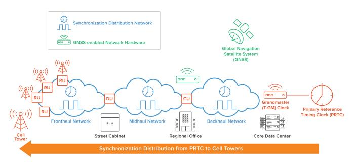
Figure 1: Simplified synchronization network
