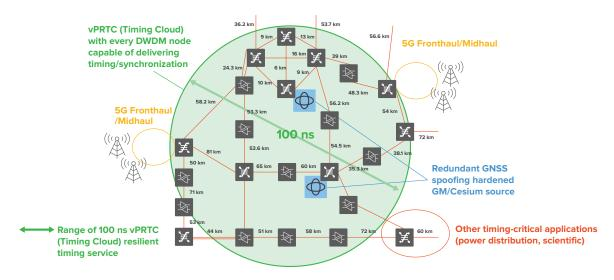
Figure 18: OTC2.0-enabled vPRTC regional/core network preserves G.8271.1 network limits for fronthaul and midhaul packet optical networks and other timing-critical applications
