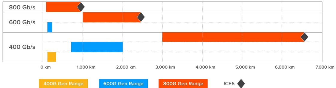
Figure 16: ICE6 capacity-reach comparison
