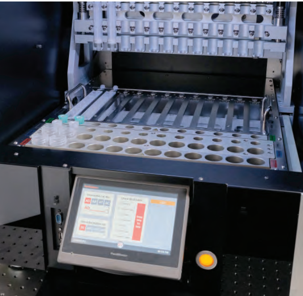
iCATCHER can perform liquid biopsy and extraction of circulating free nucleic acid. The maximum sample volume is 4,000µl of serum and the minimum elution volume is 30µl. It can obtain circulating free nucleic acid with high concentration and purity, becoming a new method for precision medicine.
