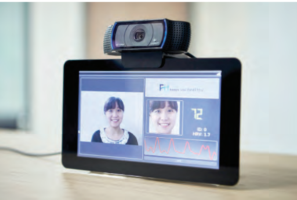
The key to this technology is detecting changes in the color of facial capillaries; it only takes 6 seconds to detect a heart rate.
