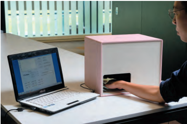
Vibrasee, a micro-vibration detector, uses a non-invasive method along with optical projection, image processing, and AI-driven data analysis technologies to detect PD. The accuracy of the detector is expected to increase to more than 90%, from 80%, in the following two years.
