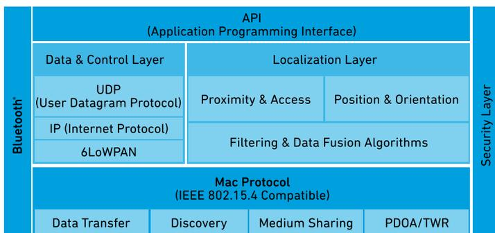
**FIGURE 2-8:** Qorvo's example of a UWB software stack.
