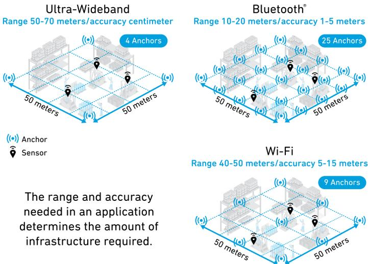
**FIGURE 1-3:** Comparing the UWB, Wi-Fi, and Bluetooth anchors required for a typical factory floor.
