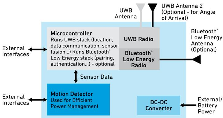
**FIGURE 2-7:** A typical UWB architecture for anchor and tag.
