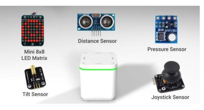
Using the included 5-pin connector, advanced learners can also interface GENIBOT with a wide range of external components to learn in a hands-on way how a robot perceives its environment. Connection possibilities include: Arduino sensors, joysticks, servo motors, ultrasound distance sensors and a micro:bit, among many other options. The sky's the limit!
