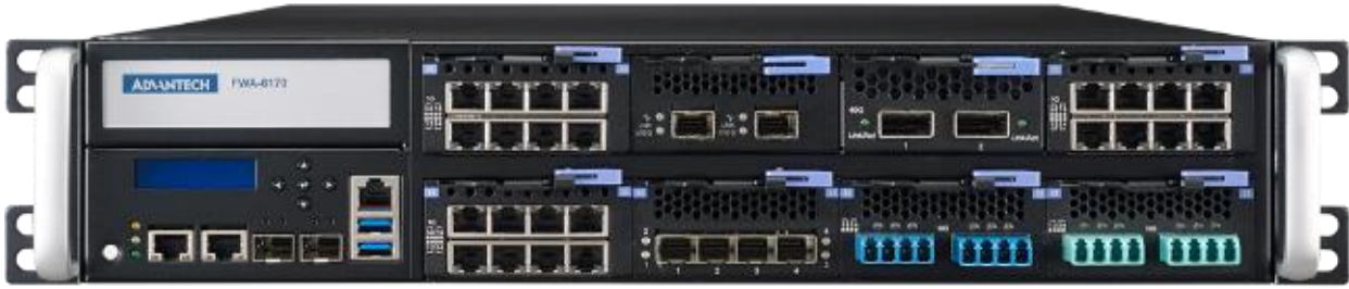
Figure 4. Advantech FWA-6170 high-end network appliance
