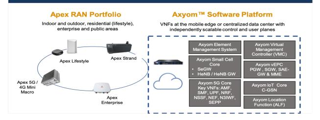
Delivering high performance with minimum power consumption and smooth integration with existing Radio Access Network (RAN), the Apex Enterprise small cell is ideally suited for network densification while also supporting VoLTE, IoT and QoS based services.
